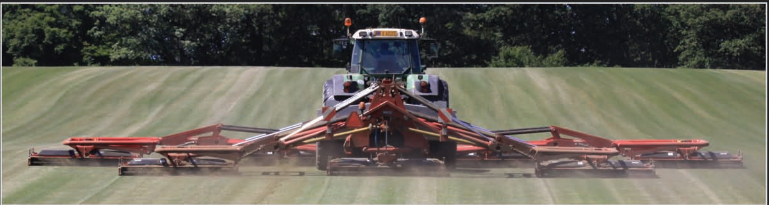
Height adjustment, infinite number of adjustments available from 1/2" to 4". All locations are fully accessible.
